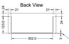
The bottom of drawer body is 3mm above the bottom
